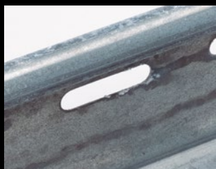
Acabado HR a 3000 horas HR coating at 3000 hours
